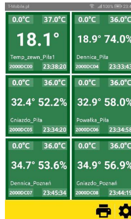
Figure 4. The phone application for monitoring temperature and humidity of the beehive.
