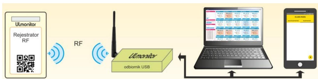
The collection of data from loggers is carried out by radio. Using the ULradio Mobile application for smartphones or (optionally) the ULradio program for a PC, the parameters are observed directly on the screen, but without the possibility of recording or archiving. It is also possible to work at B1 level provided that the loggers are placed in a right place in the hive so that the data can be downloaded contactlessly via NFC.
