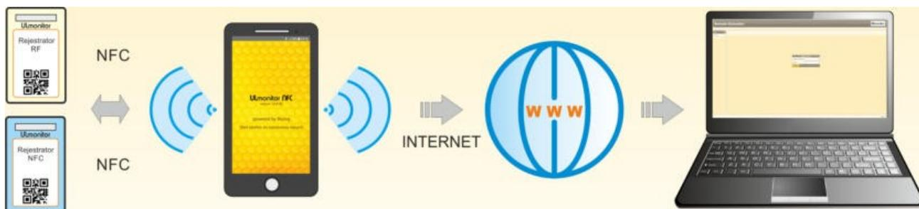
In order to continue the data recording (with 10-minute recording periods), readings should be taken at least once a month. After logging in, the console allows full control over the loggers from any place and any computer or telephone. If you do not have access to the internet, it is possible to work on level B1. If you have radio loggers in addition to NFC loggers, you can also read them on A2 level (you need an additional USB data receiver for your phone plus the ULradio Mobile application).
